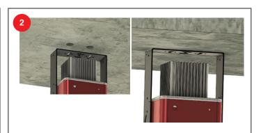
Then affix the Virtualine™ LED THIN to your mounting surface using hardware designed for that type of mounting surface (drywall anchors for drywall without a stud, concrete screws for concrete). Once the fixture is in place, clear any dust or debris out of the rear heatsink area before powering on the fixture.
