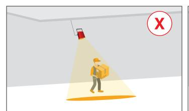
**WALL MOUNTING** This mounting type will distort the line projection to an elliptical shape – thicker in the middle, thinner at the edges.
