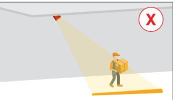
**OFFSET MOUNTING** This mounting type will distort the line projection to a conical shape – thinner closest to the units, wider it moves away. Also, the line intensity will scale brighter to fainter as you move further away.
