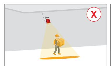
**WALL MOUNTING** This mounting type will distort the line projection to an elliptical shape – thicker in the middle, thinner at the edges.
