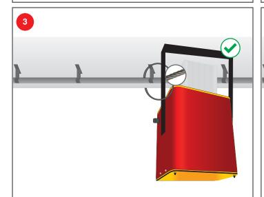
Finally, be sure to loop the included steel safety cable through the eyelet on the back of the Virtualine™ LED PRO and around the nearest secure object, pipe, or rail. This is to prevent injury in the unlikely event that the primary mount fails.
