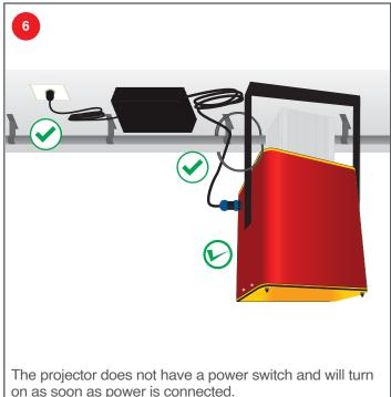
**NOTE:** When installing the power supply, do not add cable extensions between the power supply and the light fixture. The length of cable between the power supply and fixture should be as short as possible (6 feet maximum, 3 feet or less
