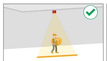
**IDEAL MOUNTING** Unit should be mounted perpendicular to the surface exactly midway of the desired projected length. E.g. if the unit produces a 20ft line from the defined mounting height, the unit should be mounted 10ft away from the start of the line
