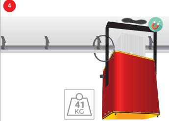
If you purchased the magnetic mount accessory, your mounting bracket will already have the magnets installed. Simply stick the magnets to the desired surface and loop the included steel safety cable around the attachment point to prevent the fixture from falling if the magnets fail. The magnets hold with approximately 90 pounds (41 kg) of force.
