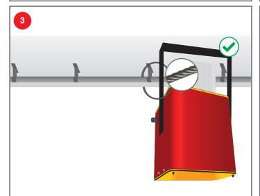
Finally, be sure to loop the included steel safety cable through the eyelet on the back of the Virtualine™ LED FILL and around the nearest secure object, pipe, or rail. This is to prevent injury in the unlikely event that the primary mount fails.
