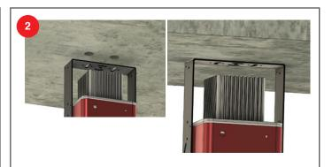
Then affix the Virtualine™ LED FILL to your mounting surface using hardware designed for that type of mounting surface (drywall anchors for drywall without a stud, concrete screws for concrete). Once the fixture is in place, clear any dust or debris out of the rear heatsink area before powering on the fixture.
