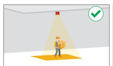
**IDEAL MOUNTING** Unit should be mounted perpendicular to the surface exactly midway of the desired projected length. E.g. if the unit produces a 20ft walkway from the defined mounting height, the unit should be mounted 10ft away from the start of the walkway.
