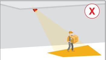
**OFFSET MOUNTING** This mounting type will distort the walkway projection to a conical shape – thinner closest to the units, wider it moves away. Also, the walkway intensity will scale brighter to fainter as you move further away.
