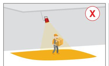
**WALL MOUNTING** This mounting type will distort the walkway projection to an elliptical shape – thicker in the middle, thinner at the edges.
