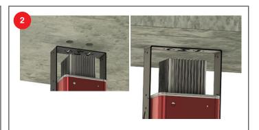
Then affix the Virtualine™ LED EDGE to your mounting surface using hardware designed for that type of mounting surface (drywall anchors for drywall without a stud, concrete screws for concrete). Once the fixture is in place, clear any dust or debris out of the rear heatsink area before powering on the fixture.
