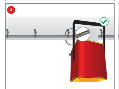
Finally, be sure to loop the included steel safety cable through the eyelet on the back of the Virtualine™ LED DOTS and around the nearest secure object, pipe, or rail. This is to prevent injury in the unlikely event that the primary mount fails.
