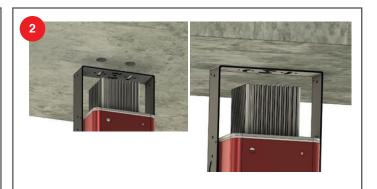
Then affix the Virtualine™ LED DOTS to your mounting surface using hardware designed for that type of mounting surface (drywall anchors for drywall without a stud, concrete screws for concrete). Once the fixture is in place, clear any dust or debris out of the rear heatsink area before powering on the fixture.
