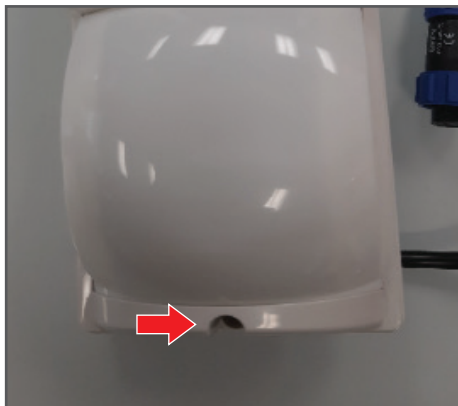
1: Unscrew the top cover of the sensor by unscrewing the screw
