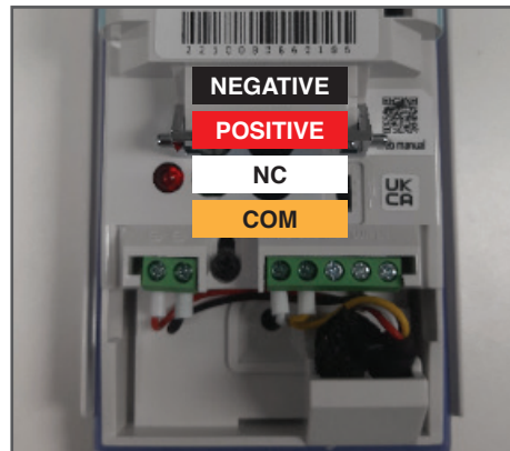
2: Remove the wires. Ignore this step if the installation space is accessible and wires do not make the installation difficult.
