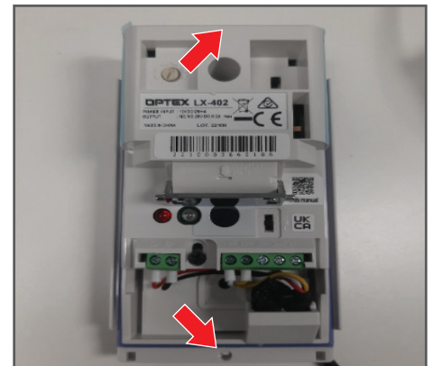
3: Use the holes to mount the bottom part of the housing on any flat surface. Screw in the wires back to the terminal block and slide in the top cover and screw it up with the screw.
