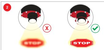
Focus the projection by threading the lens in and out until the image is well focused. The projector is shipped with the lens all the way retracted to reduce the overall size. You may need to unscrew the lens more than 40 complete revolutions before good focus is achieved.
