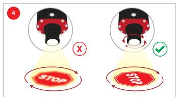
Re-adjust the focus if necessary. Note that the **image rotator** is **not** intended for continuous operation. Damage to the image rotator resulting from continuous use is not covered under warranty.
