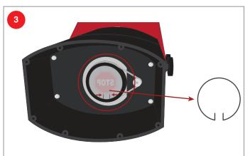
Push the two pins of the image template retaining ring together and pull out the retaining ring.
