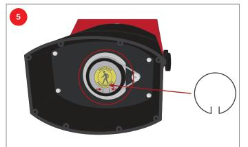
Replace the retaining ring and make sure it evenly pushes the image template all the way in.
