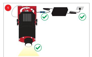
The projector does not have a power switch and will turn on as soon as power is connected.
