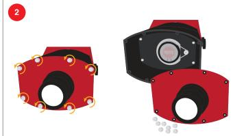
Remove the front cover (with the projection lens) by removing the eight screws holding it in place.
