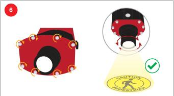
Replace the front cover and adjust the focus as needed. You will likely need to use the image rotator to align the projection as well.
