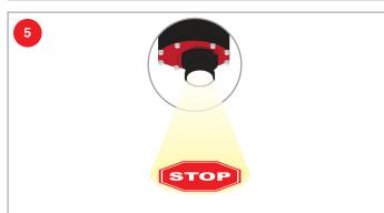
The focus can be locked in position by tightening the retaining ring on the focusing lens onto the projector body. Note that there is a rubber O-ring to prevent the retaining ring from damaging the projector.
