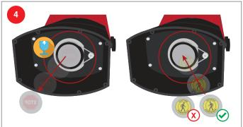
Carefully remove the old image template and replace it with the new image template. The image template should appear to be backwards or mirrored when looking into the front of the projector.
