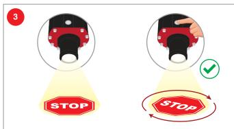
Turn on the image rotator with the pushbutton on the side of the projector, and switch it back off when the image projects in the desired position. There are no controls for speed or direction of the image rotator.
