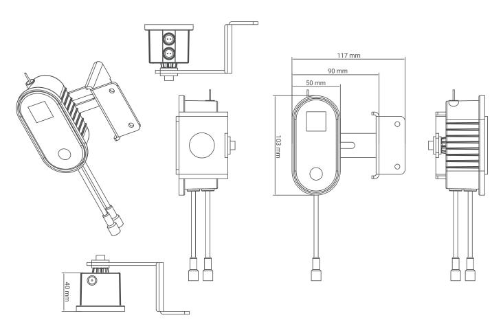
Mount the bracket to the center of the forklift carriage, aligning so that the laser module is approximately level with the top of the forklift's tines.
