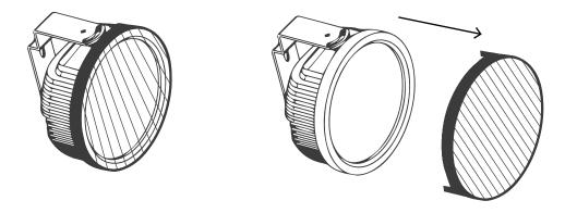
To project a SPOT, remove the lens cap manually.
